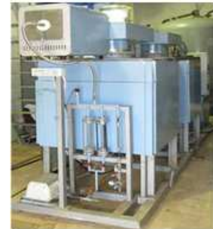
Pilot plant for oxidation of reactor graphite in molten salts for removal of contamination due to spent fuel debris
