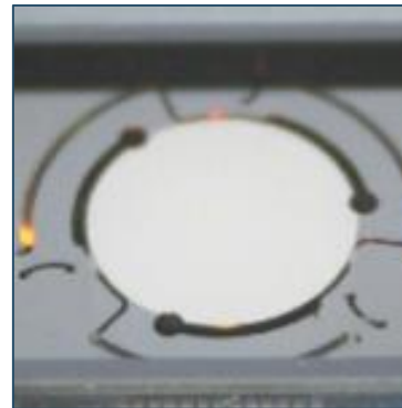
Formation micro scanners (or MEMS mirrors) Diameter 1-2 mm
