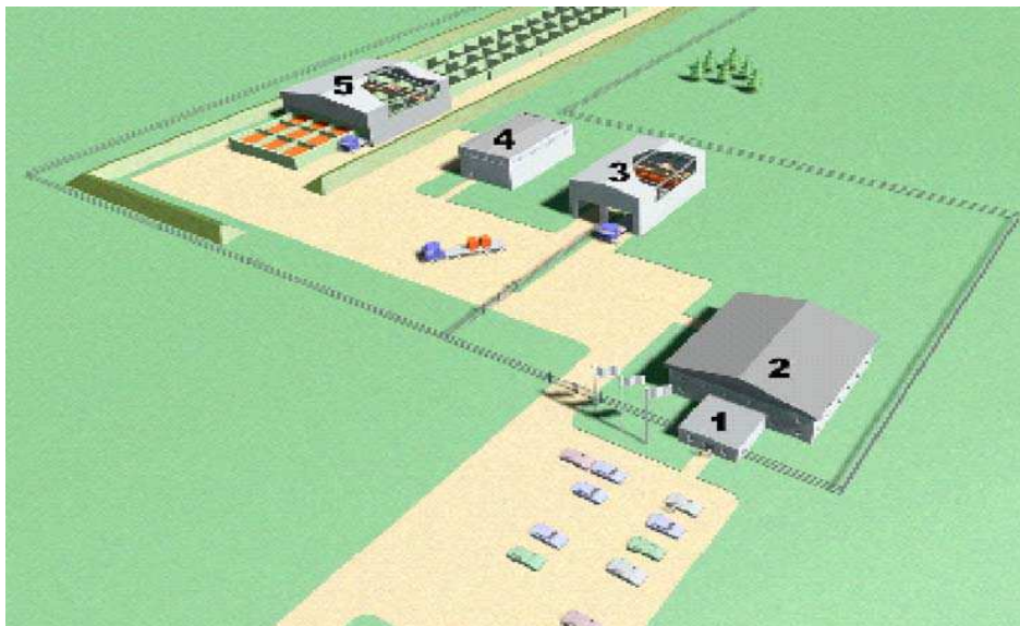
Fig. S.2. Possible layout of the near surface repository (will be adjusted to specific site in the design stage): 1 – entrance, security check; 2 – administration, central control room and laboratory; 3 – interim (buffer) storage of radioactive waste packages; 4 – facility for service systems and equipment; 5 – waste disposal area and a shelter.
