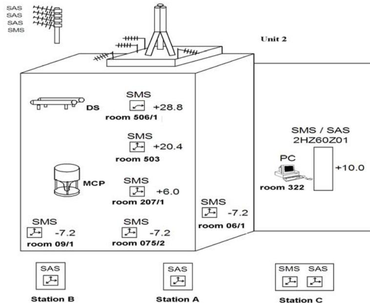
**Figure 8.1-2.** Layout of the Seismic Equipment at the INPP
