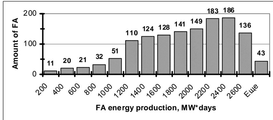
**Figure 8.3-2.** Distribution of the SFA in the Reactor according to the Energy Production
