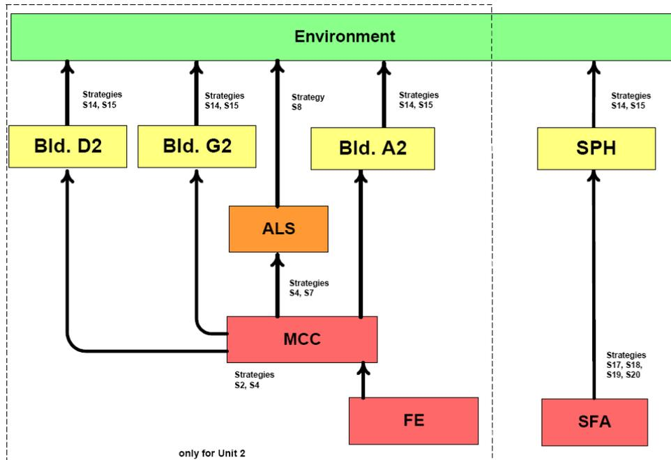
**Figure 8.4-2.** Diagram of the possible ways of the radioactive fission products emission and beyond design-basis accidents management strategies at INPP
