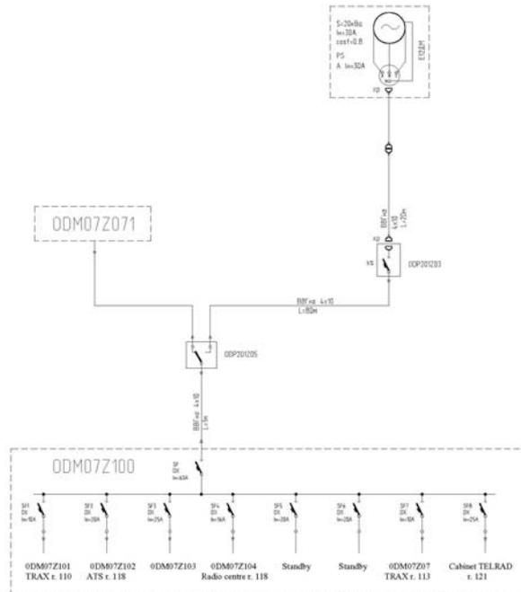
**Figure 8.4-8.** Emergency power supply circuit from mobile diesel generator VS-184E to Building 185
