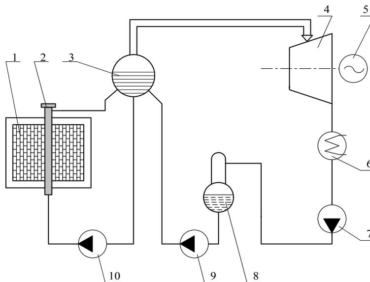
**Figure 7.3-1.** Simplified INPP heat diagram
