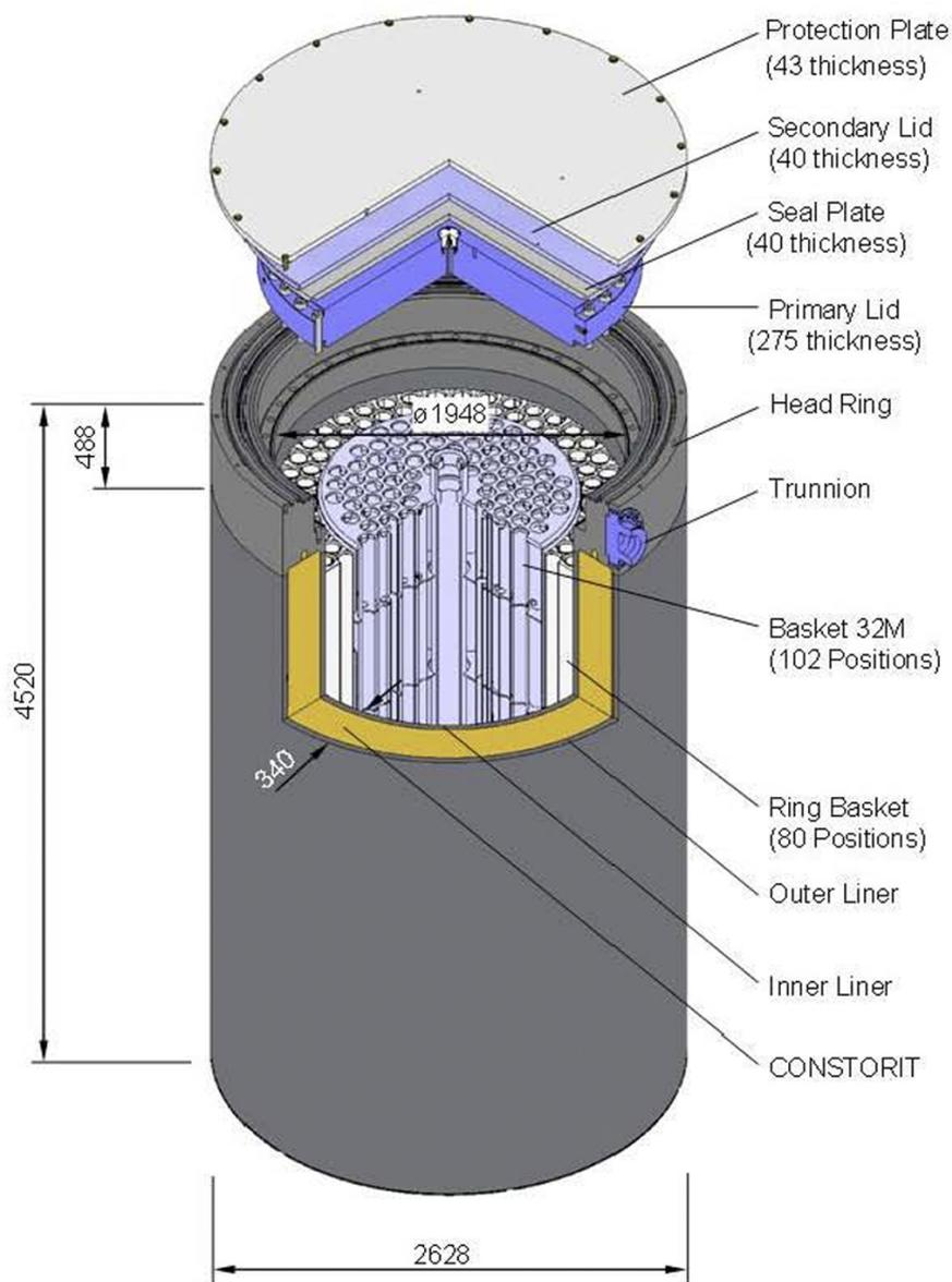
**Figure 7.8-2.** General view of CONSTOR<sup>®</sup> RBMK-1500/M2 cask with 32M basket and ring basket without concrete lid
