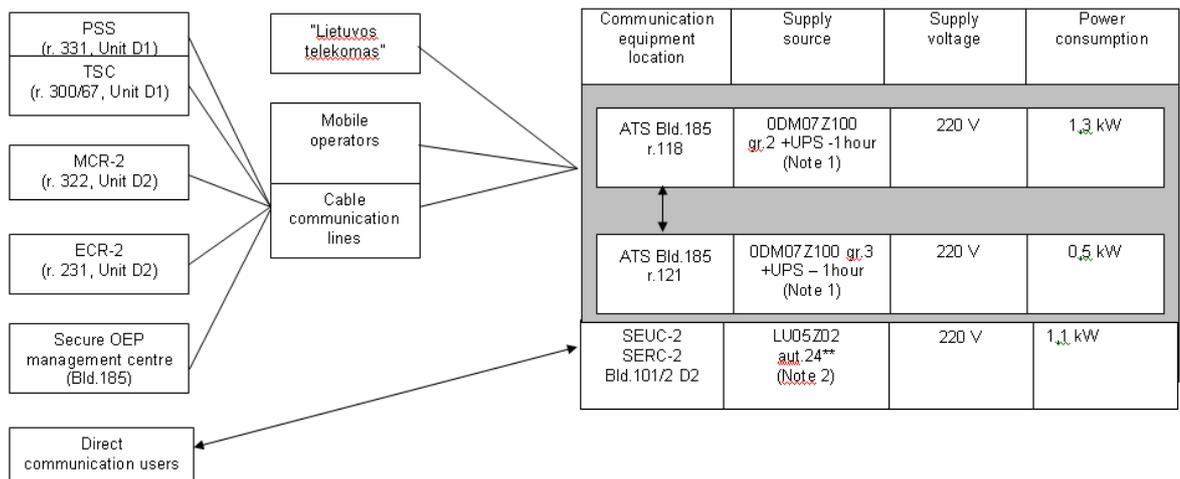
Note 1. Power supply from mobile DG with capacity 16 kW, located at Bld.185 (Bld.185 automatic telephone systems operability is supported).
