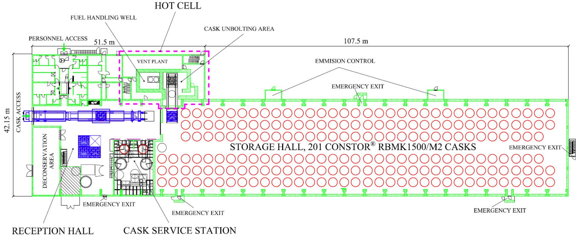
Figure 7.8-1. ISFSF main building plan
