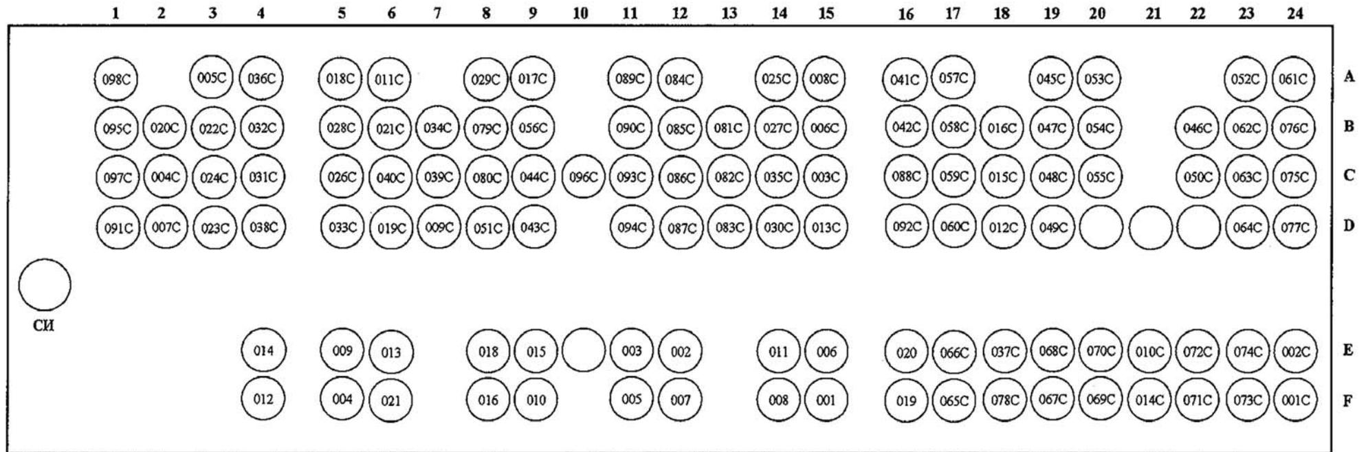
Figure 7.7-3. Cartogram of SNF casks layout at the DSFSF site as of 1 July, 2011
