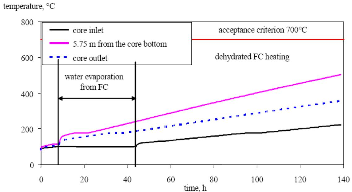
**Figure 8.3-4.** Change of FE claddings temperature at emptying of FC in 365 days after the reactor shutdown
