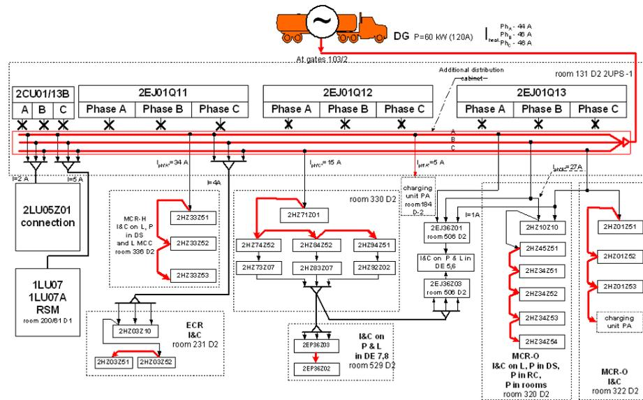
Figure 8.4-7. Emergency power supply 0.4 kV circuit from mobile diesel generator DES-60R to Building 101/2
