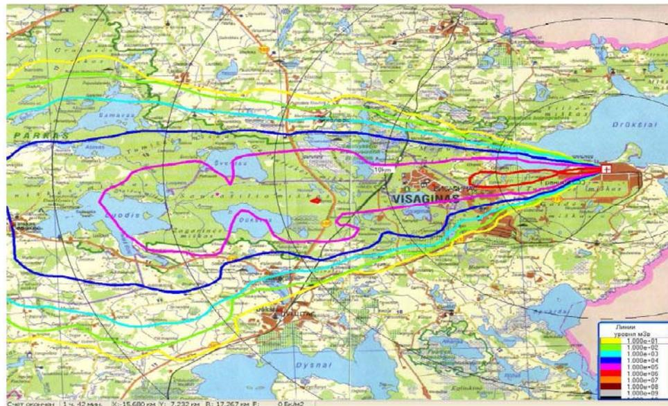
**Figure 8.4-16.** The SE INPP surroundings map with the plotted lines of the level of the district radioactive contamination from the radioactive emissions
