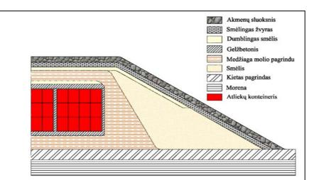
Boulder/pebbles Sandy gravel Silty sand Reinforced concrete Clay based material Sand Firm basis Glacial till Waste cask Fig. 2.4.1. Cross-section of the vault after the closure of the repository (*Reference Design ..., 2002*).
