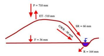
Fig. 4.1.1.6. Summarised water balance in the Apvardai site: P - atmospheric precipitation, ET - evaporation, SR - surface run-off, GWR - groundwater run-off to rivers and drains, and R - outflow.
