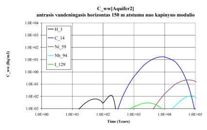
(antrasis vandeningasis horizontas 150 m atstumu nuo kapinyno – the second aquifer at a distance of 150 m from the repository module)
