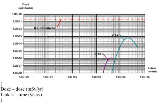
Picture 4.3.2.8. Effective doses (depending on time), caused by radionuclides migration for the site of Apvardai according to natural development scenario when contaminated groundwater gets into Apvardai lake, and their comparison with the annual dose constraint equal to 0.2 mSv.
