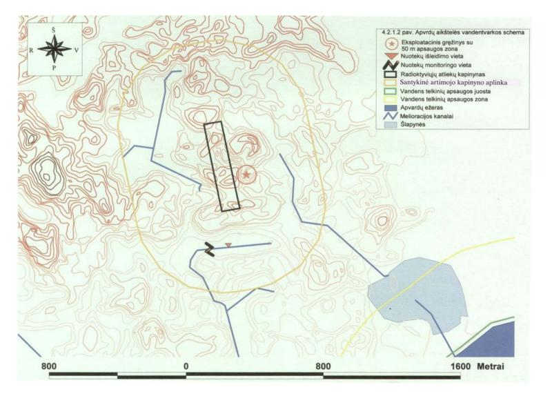
Picture 4.2.1.2 Water Supply Management Scheme at Apvardai Site. Legend definitions (from top down): a) exploitation bore with a 50 meter protection zone; b) waste water discharge site; c) waste water monitoring site; d) radioactive waste repository; e) relative surrounding repository environment; f) water basins protection strip; g) water basins protection zone; h) Apvardai Lake; i) irrigation channels; i) wetlands
