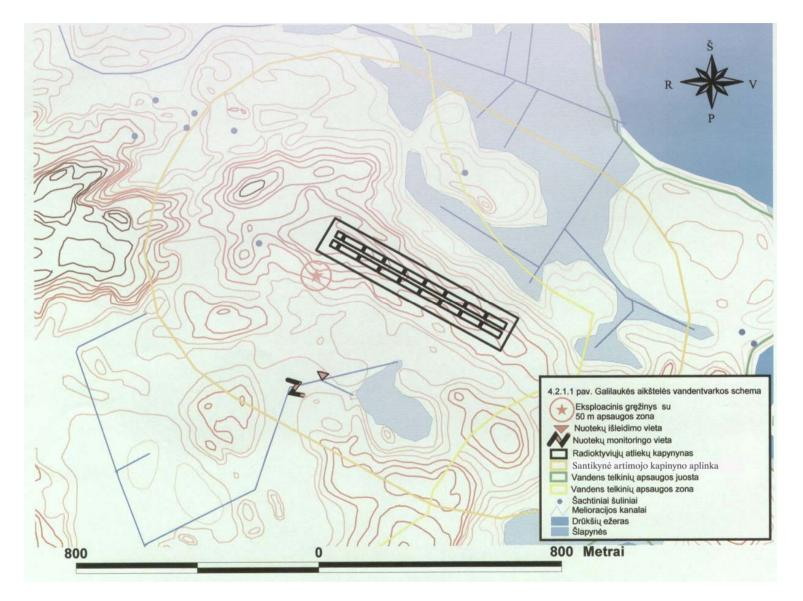
Picture 4.2.1.1 Water Supply Management Scheme at Galilauke Site. Legend definitions (from top down): a) exploitation bore with a 50 meter protection zone; b) waste water discharge site; c) waste water monitoring site; d) radioactive waste repository; e) relative surrounding repository environment; f) water basins protection strip; g) water basins protection zone; h) shaft wells; i) irrigation channels; i) Druksiai Lake; j) wetlands
