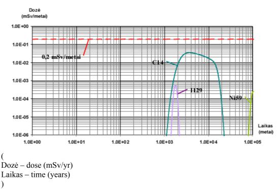
Picture 4.3.2.9. Effective doses (depending on time), caused by radionuclides migration for the site of Galilaukė according to engineering barriers degradation scenario when contaminated groundwater gets into the well drilled near the repository, and their comparison with the annual dose constraint equal to 0.2 mSv.
