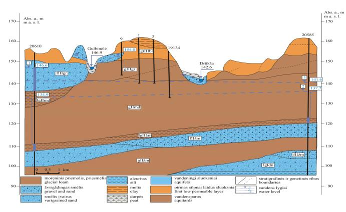
Fig. 4.1.1.4. Hydrogeological profile of the Galilaukė site and its environs, adjusted according to the study data of 2003 and 2004. Water levels: 1 – groundwater, 2 – semi-confined-confined aquifer, 3 – Lake Drūkšiai. The site of the hydrogeological profile is shown in Fig. 4.1.5.4 (C-C section of the profile between bores No. 20610 and No. 20589).
