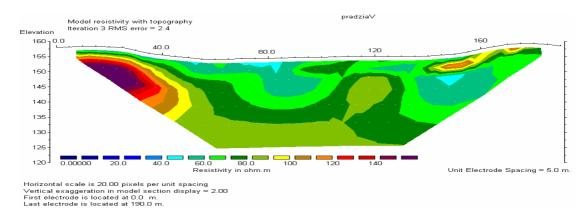
Fig. 4.1.5.10 Geoelectrical models with topography along profiles 1 and 2 at Apvardai site (see profile lines in Fig. 4.1.5.9)
