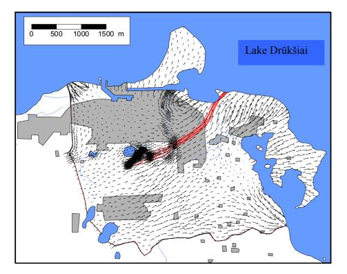
Fig. 4.1.1.15. Directions of flows of underground water of the main aquifer in the Stabatiškė site simulated using the FEFLOW code (the lines of flows from the repository site are marked in red)
