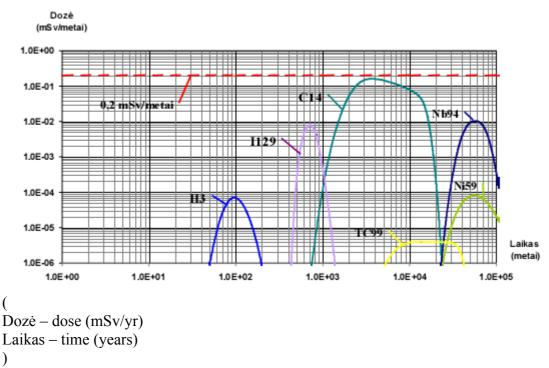
Picture 4.3.2.10. Effective doses (depending on time), caused by radionuclides migration for the site of Apvardai according to engineering barriers degradation scenario when contaminated groundwater gets into the well drilled near the repository, and their comparison with the annual dose constraint equal to 0.2 mSv.
