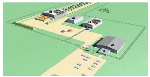
Fig. S.2. The conceptual design of the proposed near-surface repository (to be adjusted to the specific layout of the site in the detail design stage): 1 - the entrance and the security check; 2 - the administration, the central control room and the laboratory; 3 - the interim storage facility for radioactive waste packages; 4 - the facility for service systems and equipment; 5 - vaults for the final disposal of
