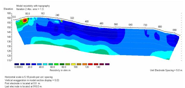
Fig. 4.1.5.15 Joint geoelectrical model with topography across the lines of profiles 1, 2, 3, and 6 (See Fig. 4.1.5.13) at Galilaukė site
