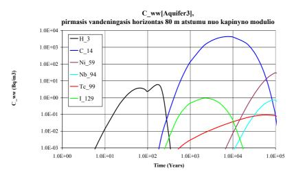
Picture 4.3.2.25. Time dependency of activities of main radionuclides in groundwater at a distance of 80 m from the repository when radioactive waste is put in casks, without placing them in containers, with clay base beneath.
