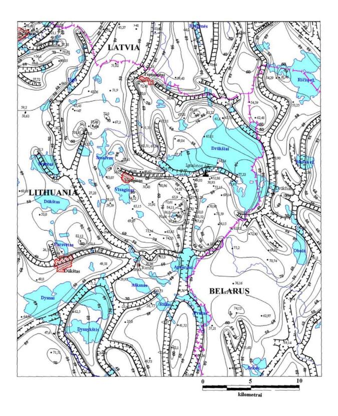
Fig. 4.1.5.3 The scheme of PostQuaternary surface of the Ignalina NPP area (Authors: *R. Kanopienė, V. Marcinkevičius*): 1 – Paleo-incisions, 2 – Isohipses of PostQuaternary surface, m; 3 – Boreholes and the absolute depth of PostQuaternary surface; 4 - Ignalina NPP.
