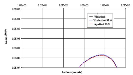
Picture 4.3.2.33. Effective doses for an adult, caused by  $^{14}$ C radionuclide, if the water from well is being consumed (the second water pathway – through the middle semi-contained aquifer; the barriers are degraded, uncertainties caused by filtration coefficient).
