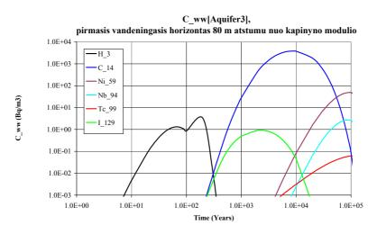
(pirmasis vandeningasis horizontas 80 m atstumu nuo kapinyno – the first aquifer at a distance of 80 m from the repository module)
