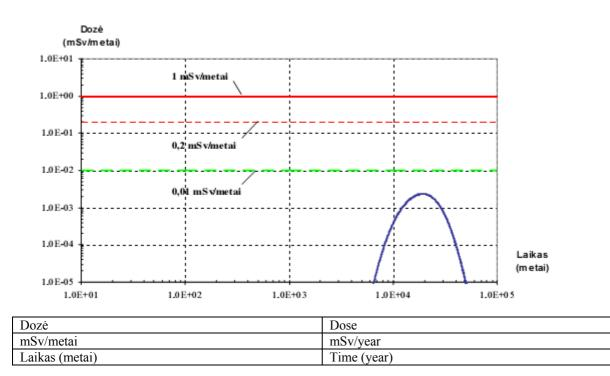
Fig. 8.4 Changes in effective doses received as a result of <sup>14</sup>C radionuclide dispersion from the Galilaukė site calculated for the scenario of degradation of repository's engineering barriers if groundwater enters a bore (well) drilled 11 km away from vaults of the repository (at the Lithuanian–Latvian border).
