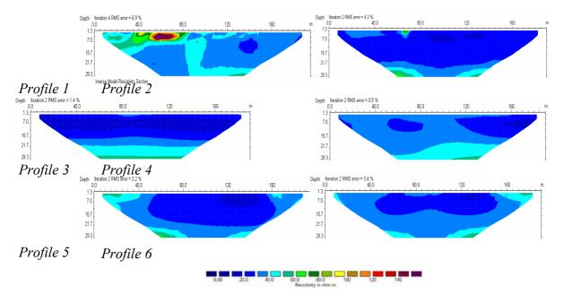
**Fig. 4.1.5.14 Geoelectrical models according to the data of electrical tomography across the profile lines 1-6 at Galilaukė site** (Numbers on the horizontal axis mean: distance from the profile beginning, on a vertical axis – depth below the land surface, at the bottom – a scale of individual electrical resistance)
