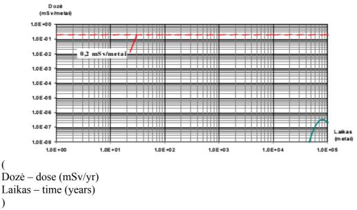
Picture 4.3.2.12. Effective doses (depending on time), caused by radionuclides migration for the site of Galilaukė, according to normal development scenario, when radionuclides are transported in the aeration zone by possible horizontal flow component and get into the well situated next to the repository.
