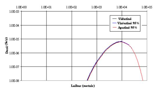
Picture 4.3.2.34. Effective doses for an adult, caused by  $^{14}$ C radionuclide through all possible exposure pathways connected to Drūkšiai lake biosphere (the second water pathway – through the middle semi-contained aquifer; the barriers are degraded, uncertainties caused by filtration coefficient).
