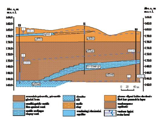
Fig. 4.1.1.7. Hydrogeological profile of the Apvardai site, adjusted according to the study data of 2003 and 2004. Water levels: 1 - groundwater, 2 - semi-confined aquifer, 3 - Lake Apvardai. The site of the hydrogeological profile is shown in Fig. 4.1.1.8.
