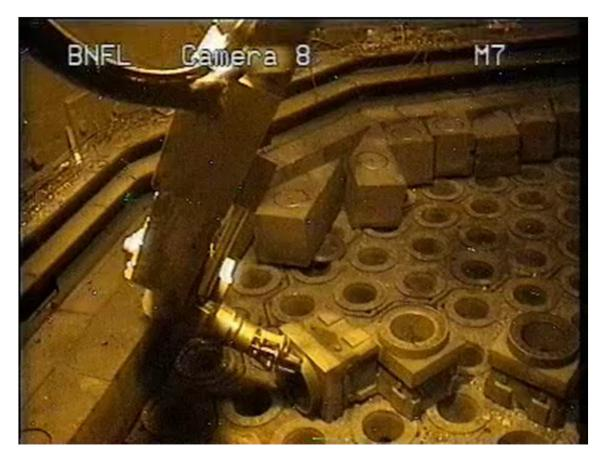
Lowest layer of core interfaces with the core support bearing top races – high dose!
