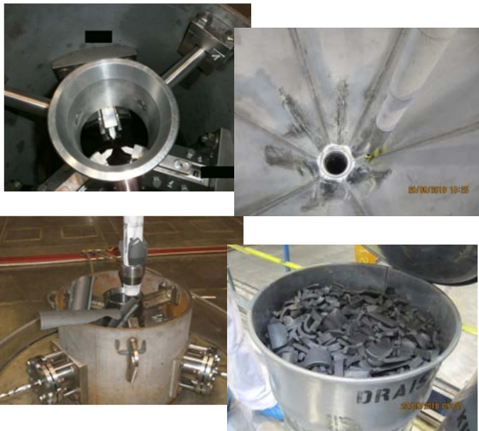
Cold tests of Graphite Crushing Device
