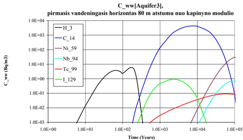
Picture 4.3.2.25. Time dependency of activities of main radionuclides in groundwater at a distance of 80 m from the repository when radioactive waste is put in casks, without placing them in containers, with clay base beneath.
