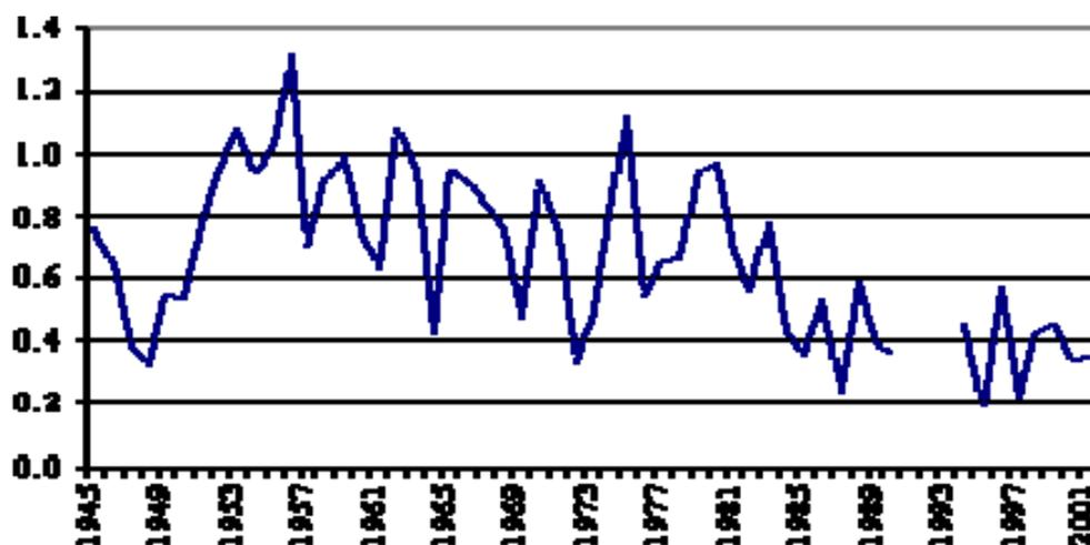
Fig. 4.1.1.1. The amplitude of water level fluctuations of Lake Drūkšiai, m. The height of 0.0 m is equal to the altitude 140.26 m.
