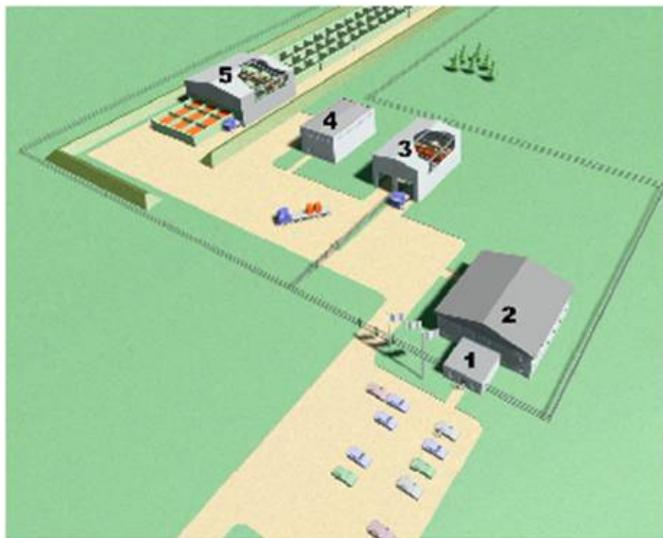
Fig. 2.3.1. The conceptual design of the proposed near-surface repository (*Reference Design ...*, 2002): 1 – the entrance and the security check; 2 – the administration, the central control room and the laboratory; 3 – the interim storage facility for radioactive waste packages; 4 – the facility for service systems and equipment; 5 – vaults for the final disposal of radioactive waste and a shelter.
