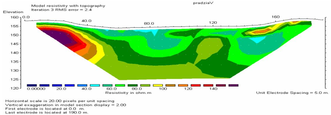
Fig. 4.1.5.10 Geoelectrical models with topography along profiles 1 and 2 at Apvardai site (see profile lines in Fig. 4.1.5.9)
