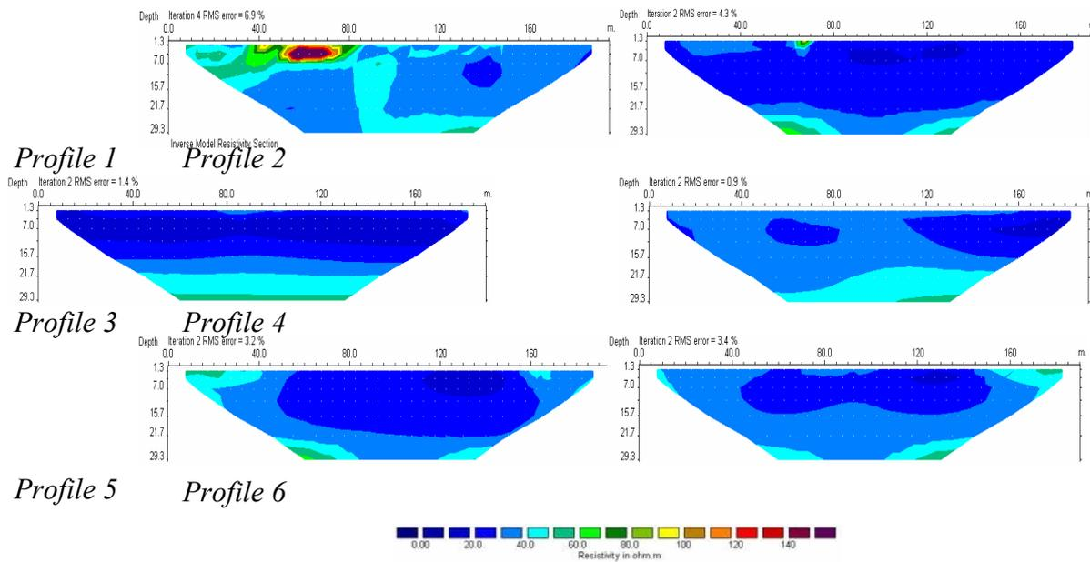
**Fig. 4.1.5.14 Geoelectrical models according to the data of electrical tomography across the profile lines 1-6 at Galilaukè site** (Numbers on the horizontal axis mean: distance from the profile beginning, on a vertical axis – depth below the land surface, at the bottom – a scale of individual electrical resistance)
