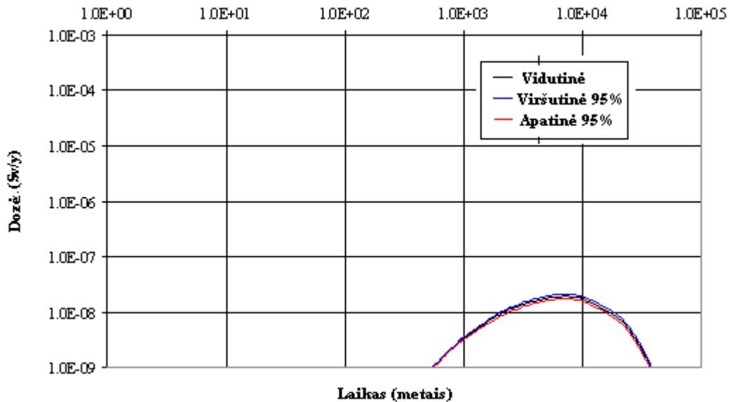
Picture 4.3.2.33. Effective doses for an adult, caused by  $^{14}\text{C}$  radionuclide, if the water from well is being consumed (the second water pathway – through the middle semi-contained aquifer; the barriers are degraded, uncertainties caused by filtration coefficient).
