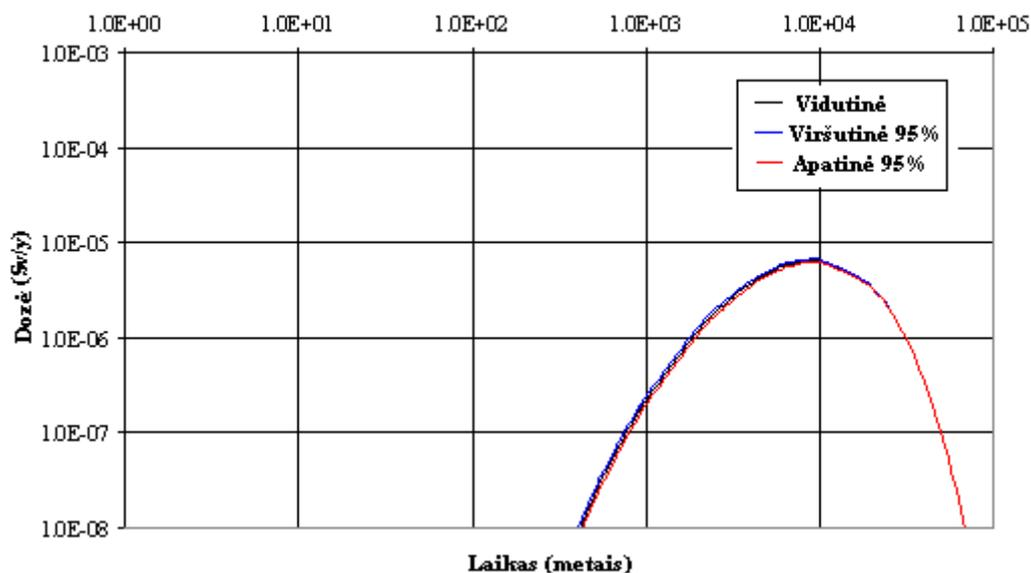
Picture 4.3.2.34. Effective doses for an adult, caused by  $^{14}\text{C}$  radionuclide through all possible exposure pathways connected to Drūkšiai lake biosphere (the second water pathway – through the middle semi-contained aquifer; the barriers are degraded, uncertainties caused by filtration coefficient).
