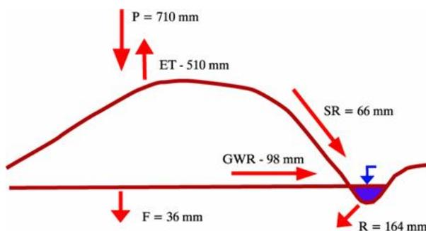
Fig. 4.1.1.3. Summarised water balance in the Galilaukė site: P – atmospheric precipitation, ET – evaporation, SR – surface run-off, GWR – groundwater run-off to rivers and drains, and R – outflow.
