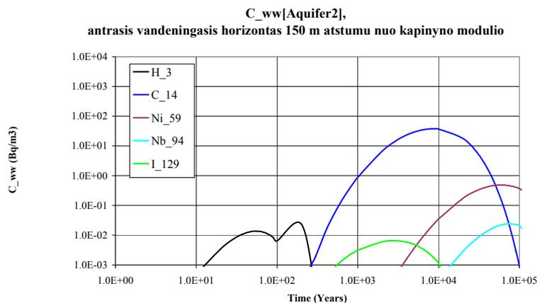
(antrasis vandeningasis horizontas 150 m atstumu nuo kapinyno – the second aquifer at a distance of 150 m from the repository module)
