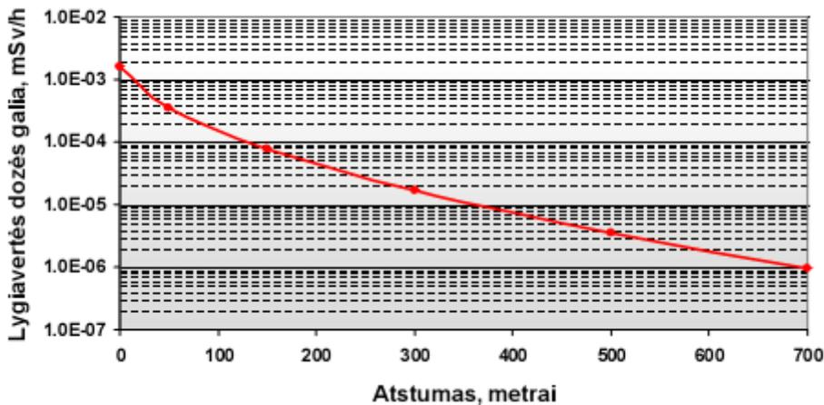
(Vertically – equivalent dose rate mSv/h; horizontally – the distance in meters)
