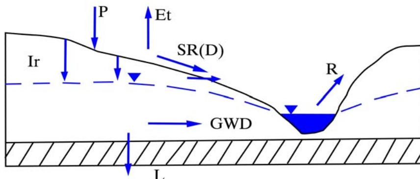
Fig. 4.1.1.10. Scheme of the water balance of the Stabatiškė site: P – atmospheric precipitation, ET – evaporation, SR – surface run-off, GWR – groundwater run-off to rivers and drains, L – crossover, and R – outflow. ( $P = 700$  mm,  $Et = 515$  mm,  $SR(D) = R = 162$  mm,  $GWD+L = 23$  mm).
