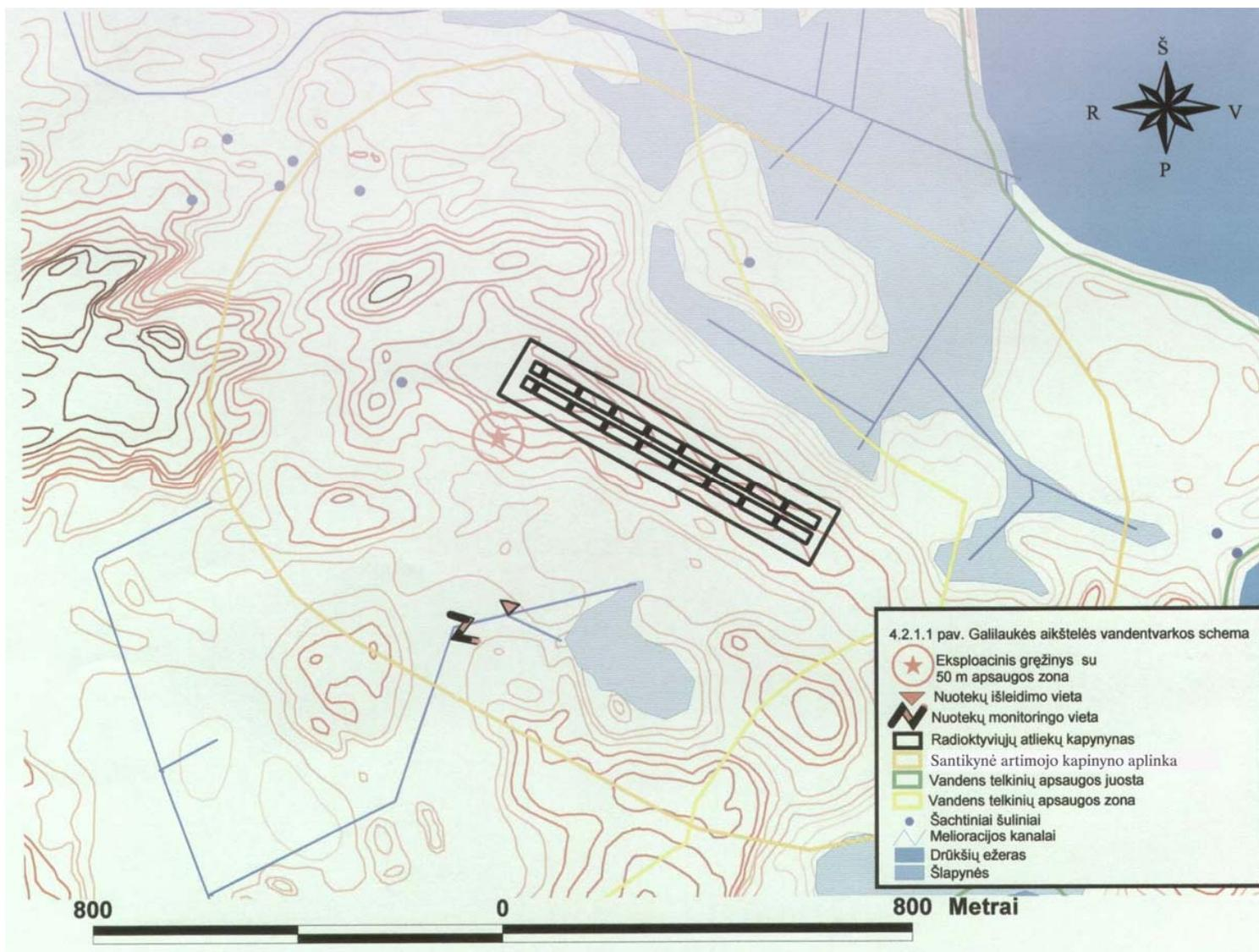
Picture 4.2.1.1 Water Supply Management Scheme at Galilauke Site. Legend definitions (from top down): a) exploitation bore with a 50 meter protection zone; b) waste water discharge site; c) waste water monitoring site; d) radioactive waste repository; e) relative surrounding repository environment; f) water basins protection strip; g) water basins protection zone; h) shaft wells; i) irrigation channels; j) Druksiai Lake; k) wetlands
