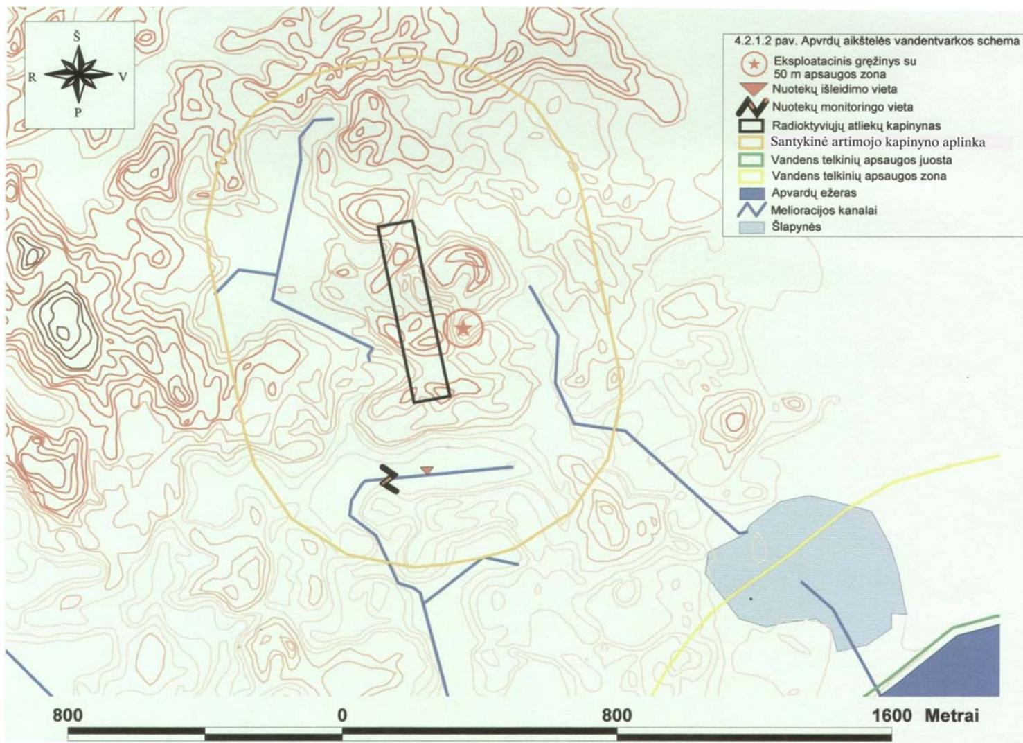
Picture 4.2.1.2 Water Supply Management Scheme at Apvardai Site. Legend definitions (from top down): a) exploitation bore with a 50 meter protection zone; b) waste water discharge site; c) waste water monitoring site; d) radioactive waste repository; e) relative surrounding repository environment; f) water basins protection strip; g) water basins protection zone; h) Apvardai Lake; i) irrigation channels; j) wetlands
