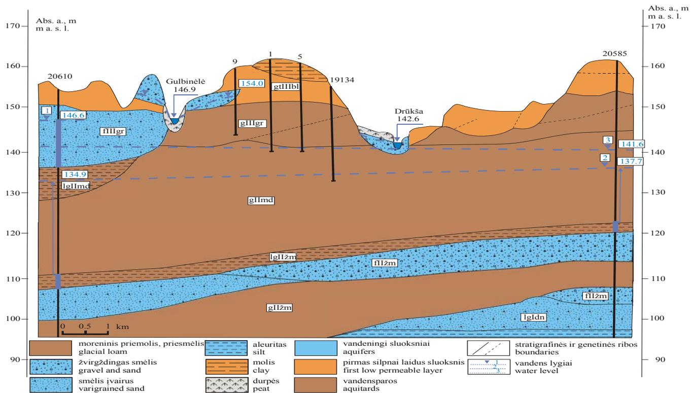
Fig. 4.1.1.4. Hydrogeological profile of the Galilaukė site and its environs, adjusted according to the study data of 2003 and 2004. Water levels: 1 – groundwater, 2 – semi-confined-confined aquifer, 3 – Lake Drūkšiai. The site of the hydrogeological profile is shown in Fig. 4.1.5.4 (C-C section of the profile between bores No. 20610 and No. 20589).
