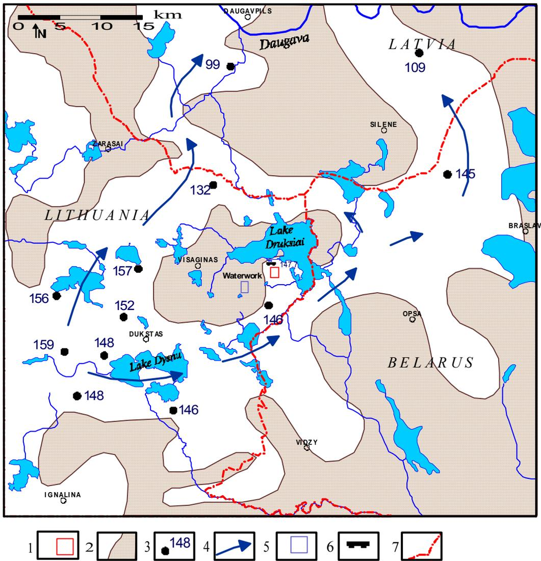
Picture 4.3.2.21. Scheme for the middle aquifer (agIII) prevalence in Ignalina NPP region: 1 – Location of Stabatiškė site in INPP region; 2 – aquifer boundary with aquitard; 3 – borehole location and groundwater level elevation; 4 – directions of water flows; 5 – area of Visaginas water intake; 6 – Ignalina NPP location in the region; 7 – the boundaries of states.
