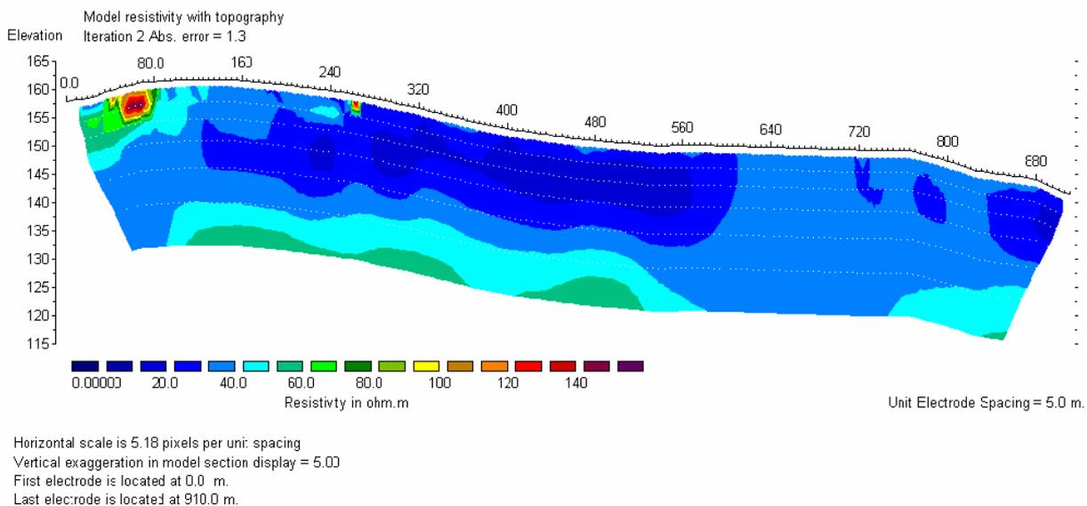
**Fig. 4.1.5.15 Joint geoelectrical model with topography across the lines of profiles 1, 2, 3, and 6 (See Fig. 4.1.5.13) at Galilaukè site**
