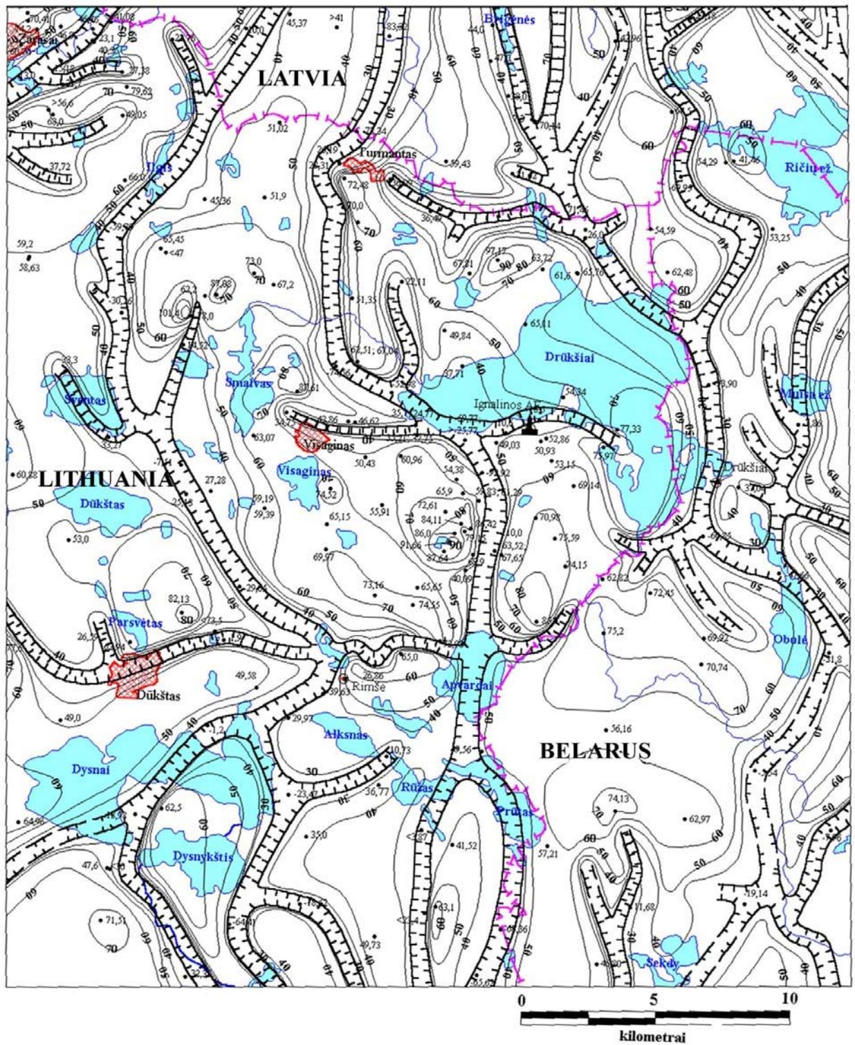
**Fig. 4.1.5.3** The scheme of PostQuaternary surface of the Ignalina NPP area (Authors: *R. Kanopienė, V. Marcinkevičius*): 1 – Paleo-incisions, 2 – Isohypes of PostQuaternary surface, m; 3 – Boreholes and the absolute depth of PostQuaternary surface; 4 - Ignalina NPP.
