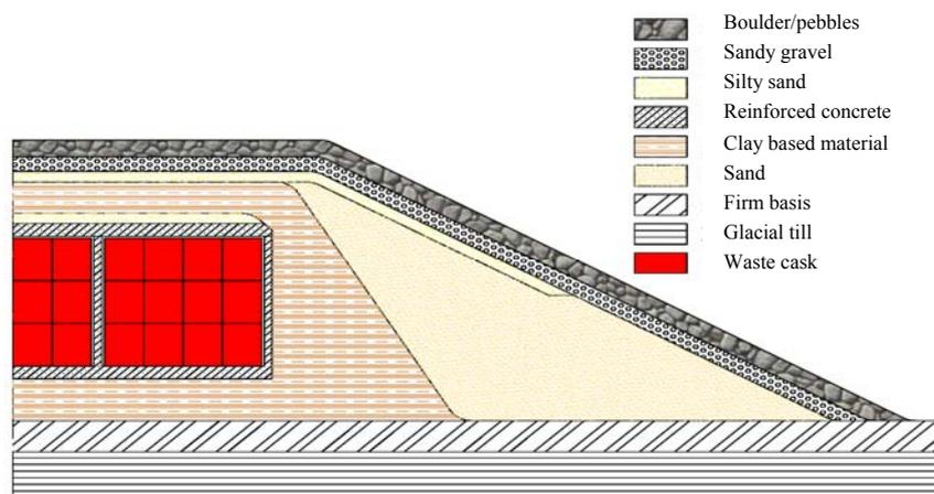
Fig. S.3. Cross-section of the vault after the closure of the repository (*Reference Design ...*, 2002).
