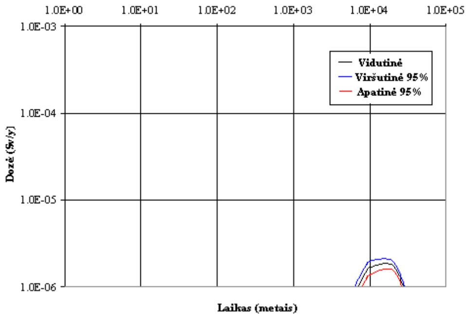
Picture 4.3.2.32. Effective doses for an adult, caused by  $^{14}\text{C}$  radionuclide through all possible exposure pathways connected to Drūkšiai lake biosphere (the first water pathway – upper aquifer and drainage system; the barriers are degraded, uncertainties caused by filtration coefficient).
