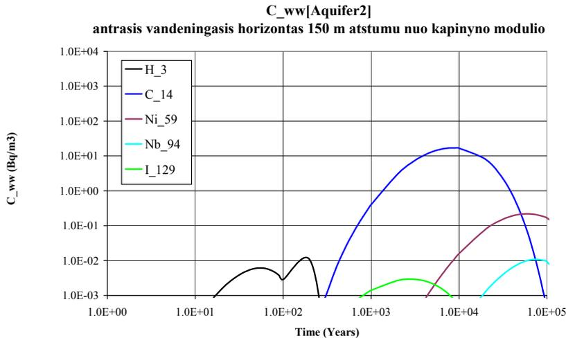
(antrasis vandeningasis horizontas 150 m atstumu nuo kapinyno – the second aquifer at a distance of 150 m from the repository module)
