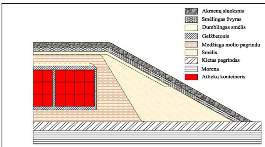
Fig. 2.4.1. Cross-section of the vault after the closure of the repository (*Reference Design ...*, 2002).
