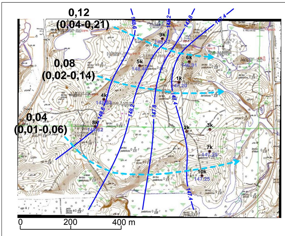
Fig. 4.1.1.14. Average altitudes of the underground water level in the Stabatiškė site (numbers provided at the bores are equivalent to the median for the total investigation period, m a.s.l.), the hydro isopiez distribution (continuous lines, m a.s.l.), water flow directions (arrows) and Darcian speed (median values and the interval of change, m/day).
