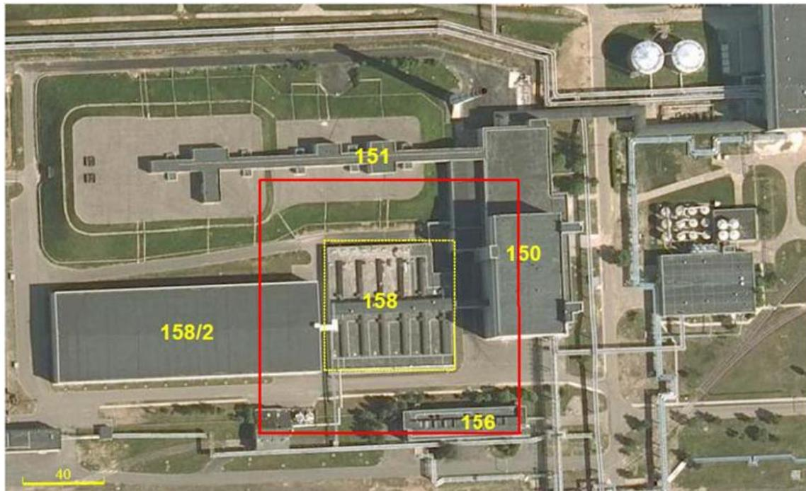
Fig. 7.2. Reconstruction of building 158 (bituminised radioactive waste storage facility) into the repository. The red line marks the 36 m wide area around the building, which will be used for the engineering barrier (multilayer cap) maintaining a slope of 3:1 [12]
