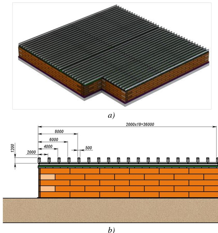
Fig. 7.3. Reconstruction of the storage facility (bld. 158) into the repository: metallic structures supporting the engineered barrier of 5.8 m thickness *a*) – general view, *b*) – cross-section [12]
