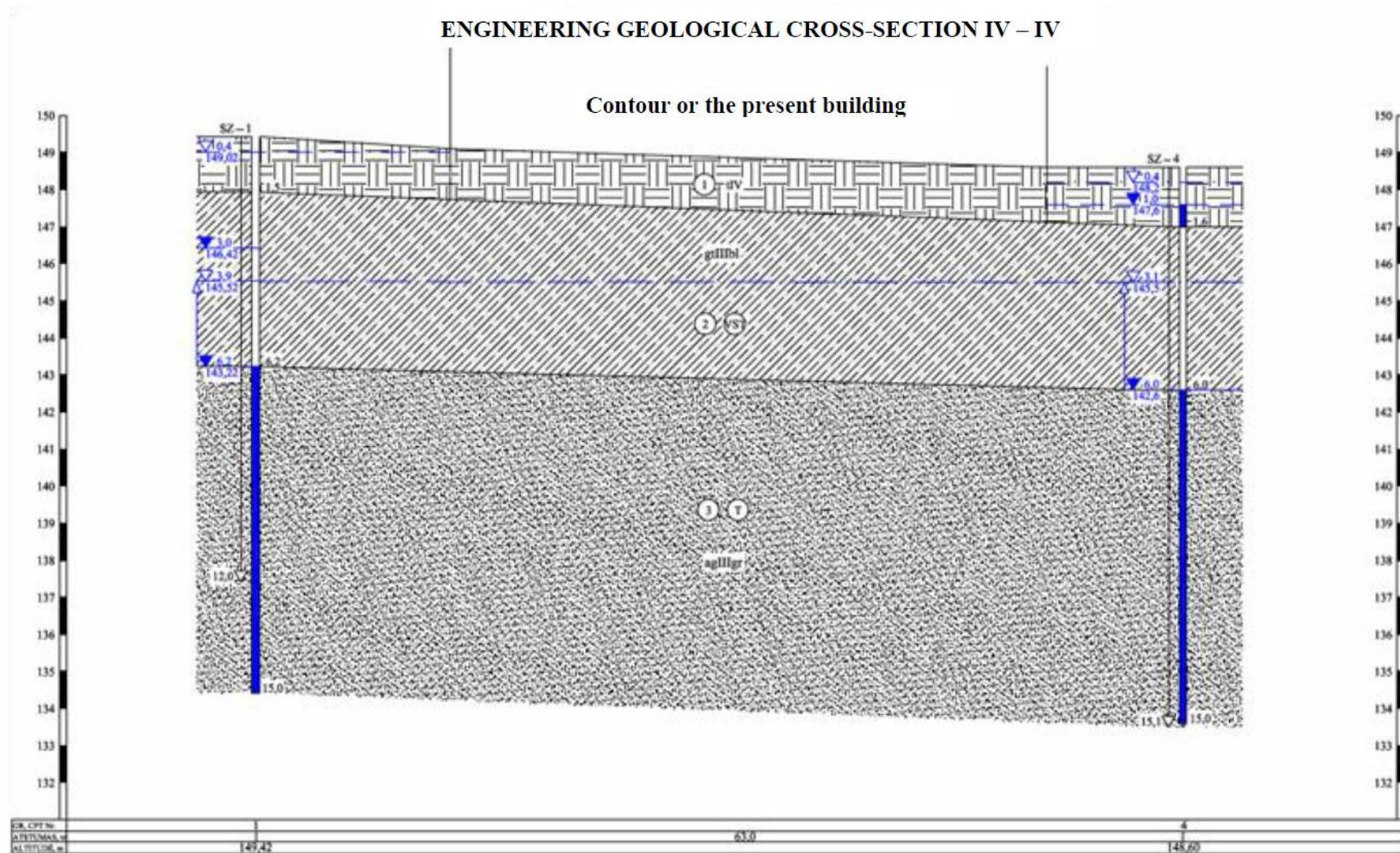
Fig. 3.8. Engineering-geological cross-sections I-I, II-II, III-III and IV-IV developed from data obtained during EGG investigations [4]
