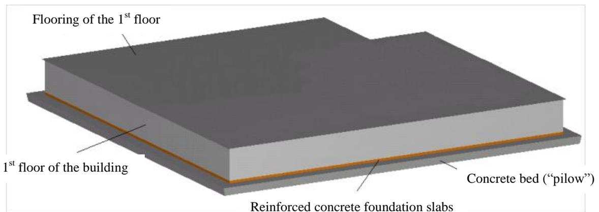
Fig. 7.1. Reconstruction of building 158 (bituminised radioactive waste storage facility) into the repository. General view of bld. 158 after the dismantling of rooms located on the second floor (simplified scheme) [12]
