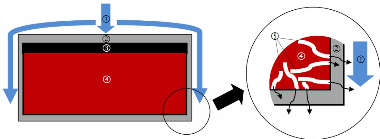
Fig. 10.2. Conceptual model of the radionuclide migration (diffusion) from the bitumen compound through the reinforced concrete structures (walls and bottom) of bld. 158: 1 – water flow; 2 – reinforced concrete structures of bld. 158 ; 3 – layer of inert material; 4 – bituminised RAW (bitumen matrix); 5 – formed pores
