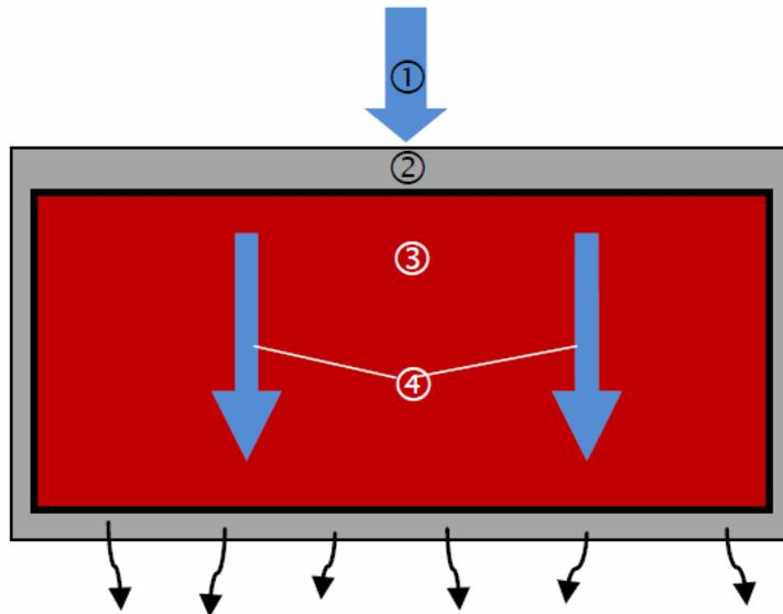
Fig. 10.3. Conceptual model of the radionuclide migration (leaching) from the sand-gravel waste through the bottom slab of bld.158: 1 – water flow; 2 – reinforced concrete structures of bld. 158 ; 3 – sand-gravel radioactive waste; 4 – diffusive-advective flow
