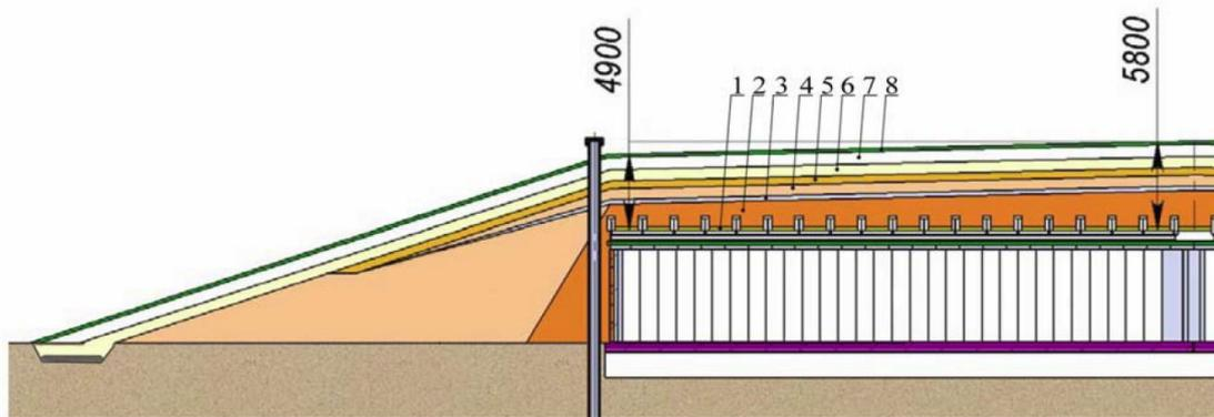
Fig. 7.4. Composition (cross-section) of the 5.8 m thick engineered barrier after transformation of the storage facility (bld. 158) into the repository:
