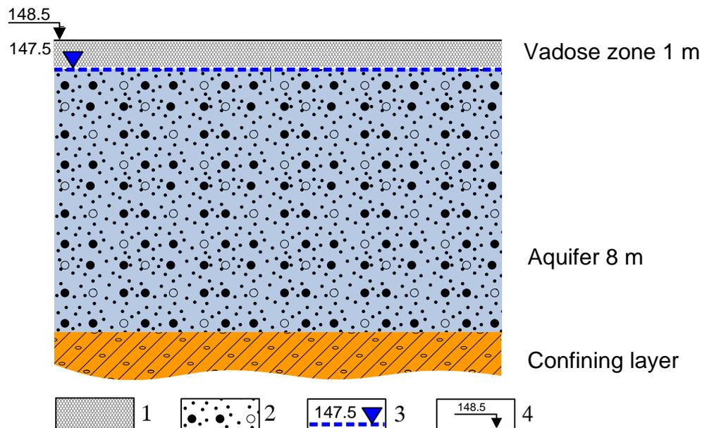
Fig. 10.1. Conceptual geological model used in the analysis:
