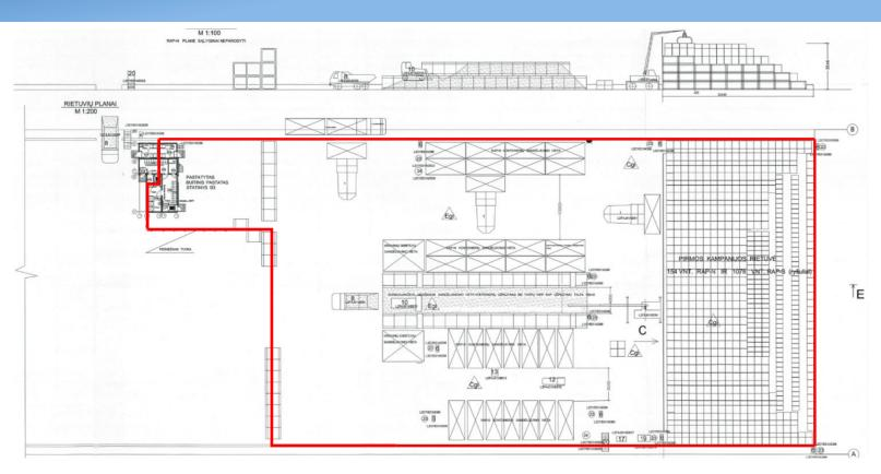
Installation of the barrier in the controlled area (the area where exposure to ionizing radiation is possible) in the form of protective wall blocks and fence sections
