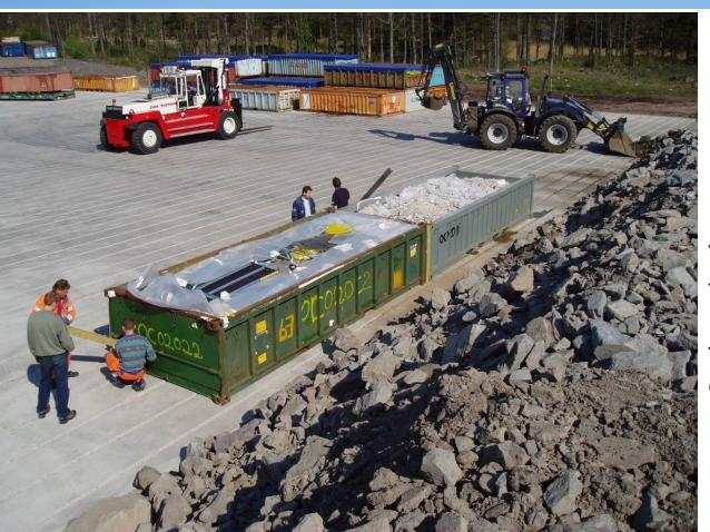
The lids are removed, and the self-adhesive tape of impregnated polyurethane foam between the containers is fixed
