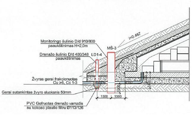
Installation of a plug into the monitoring well, as well as monitoring and drainage wells raising during the performing of work
