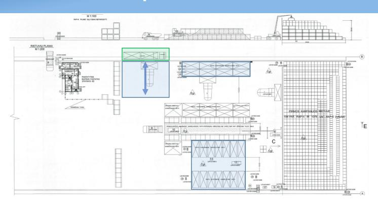
To avoid contamination, the truck with containers does not enter the radioactive waste management zone, and the forklift does not leave it.
