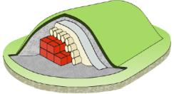
The main part of the repository is the base slab on which the radioactive waste is placed.
