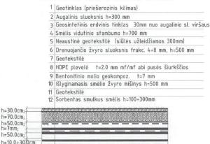
Repository cover structure, according to the design. The main layers (works) corresponds to the layers previously shown in the photos of Swedish repository
