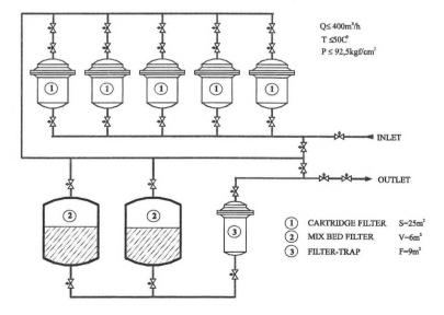
In 10 years of operation the defects were identified on the valves caused by the abrasive qualities of the applied inorganic absorbent PERLITE. Only 20% of radioactivity of corrosion products were present in the primary circuit as particles with
